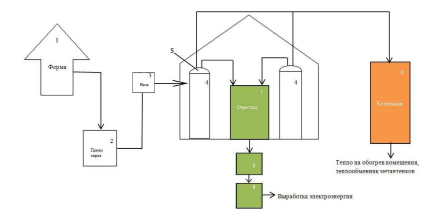
1 – farm, 2 – feedstock receiver, 3 – pump, 4 – heated digestion tank, 5 – combined gas collector, 6 – boiler room, 8 – separate gas collector, 9 – cogeneration plant
